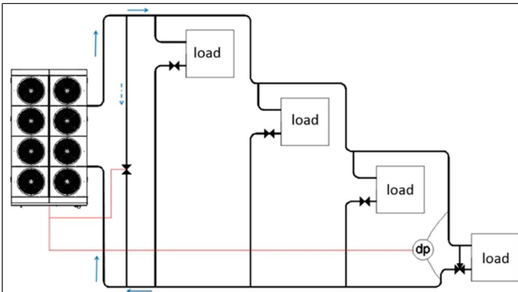
A bypass line (field supply) needs to be installed which guarantees that at all times the minimum water flow of the chiller is supplied (refer to the "Operating limit" chapter for indication on minimum water flow). The bypass valve will be an ON/OFF normally closed valve controlled by the chiller. In case the minimum water flow allowed is not reached, the chiller will open the bypass line restoring the water flow above the minimum value.
