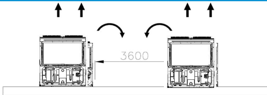
For multiple chiller installation it is recommended to install the chillers in a single row as shown in the picture below
